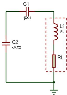
$X_L$  could be a reactance of an inductor or motion inductance of a crystal.
