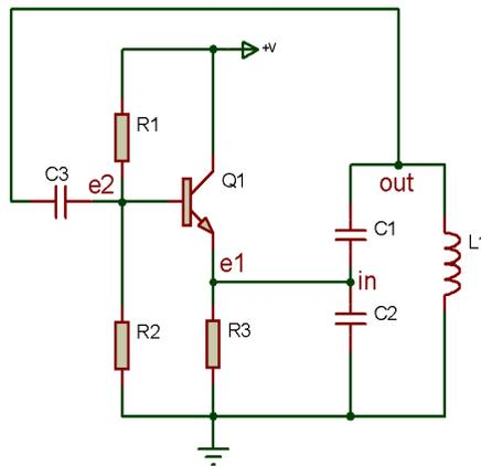
The emitter follower has a high current gain and has a voltage gain of  $< 1$ . The phase through the emitter follower will be  $0^\circ$  so the circuit should not oscillate. The gain takes place in the feedback network.
